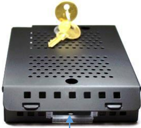
Power, GPS, Remote, Camera 1, 2, & 4 cables should go through this opening should go through this opening
